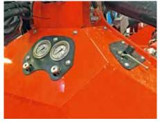
The OPTIMER 6000 and 7500 stubble cultivators are equipped with the optional STEADY CONTROL ground tracking system. It is fitted as standard on the 9 and 12 metre models for perfect control of the working depth whatever the soil conditions
