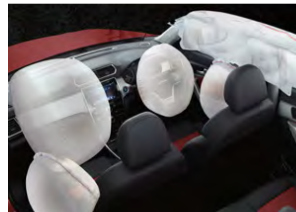
Front dual, front dual side and integrated side curtain airbags.
