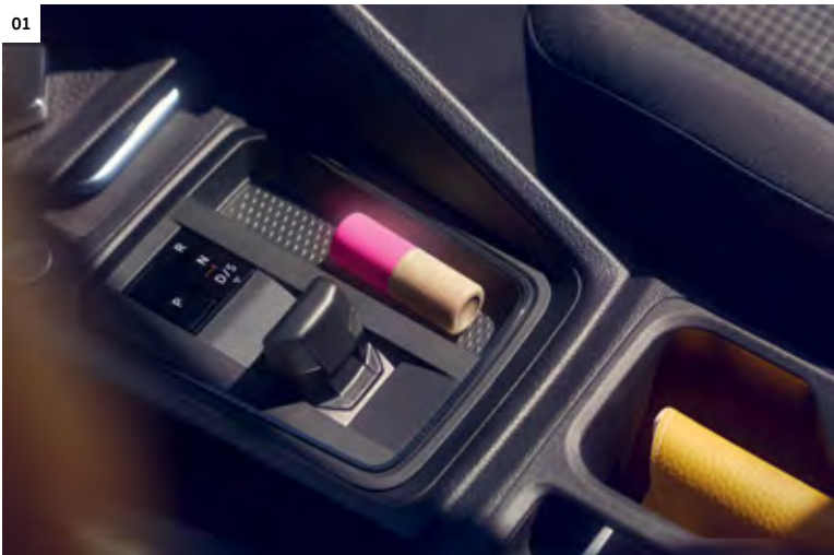
01 Dual-clutch gearbox (DSG). The new Caddy is fitted with an adaptive 7-speed dual-clutch gearbox. This enables fully automatic, smooth gear changes without interruption of tractive power, and it also adapts to the driver's driving style. You can also shift up and down using rocker switches on the steering wheel. | C | L |
