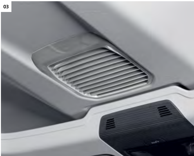
03 Comfort ventilation in the passenger compartment. The blower integrated in the roof draws in warm or cool fresh air above the instrument panel and distributes it through five vents into the passenger compartment, where it reaches the third row of seats. | C | L |
