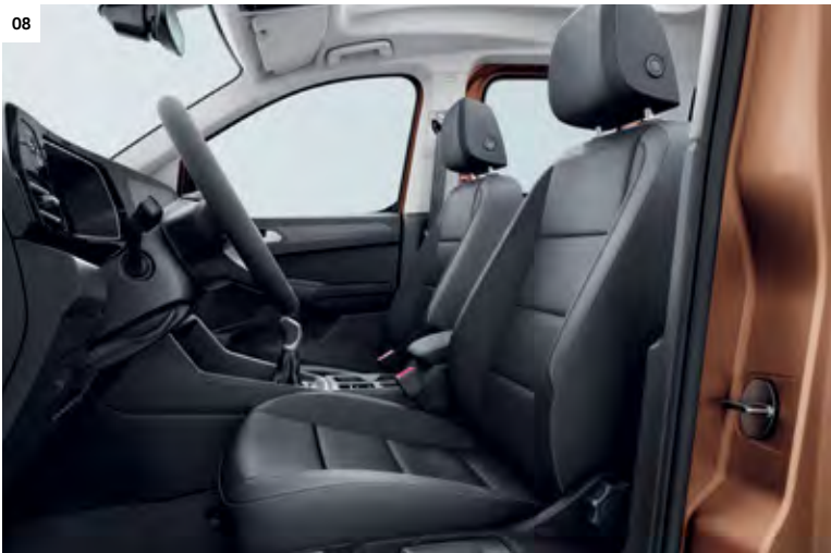
08 ergoComfort seat (AGR). The comfort seat, which has been certified as back-friendly by Aktion Gesunder Rücken (AGR) e.V.3), features a comprehensive range of settings designed to support the spine. In addition to adjustment of the seat length, seat height, seat depth, seat tilt, backrest and head restraint, the ergoComfort seat features electric 4-way lumbar support. | C | L |
