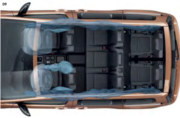
09 Front, side, curtain and centre airbags. The new Caddy is equipped with one front airbag for the driver and one for the passenger. Centre airbags prevent a collision between the driver and front passenger. And curtain airbags offer all passengers sitting on the outer seats protection in the event of a side-on collision. | C | L |
