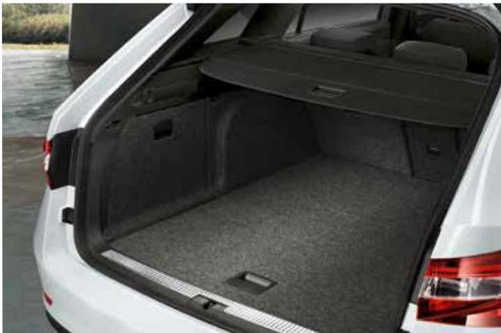
When Virtual Pedal A is equipped, the rolling cover of the luggage compartment provides shifts to the centre position after the electric tailgate is opened, making it easily accessible to luggage.
