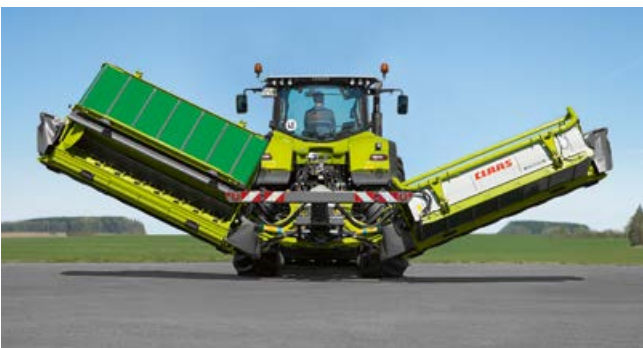
Professional control system provides individual lift and folding capability
