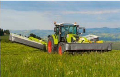
Compact headstock at the front linkage gives the mower generous ground clearance at headlands
