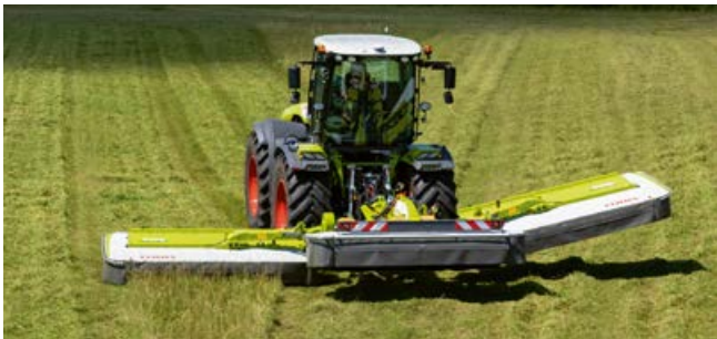
Individual mower unit lift at the headland
