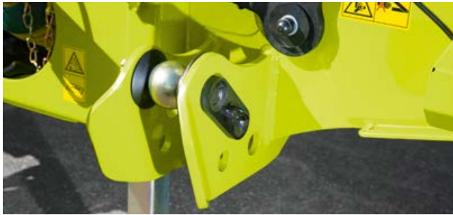
Lower link guides for ease of mounting
