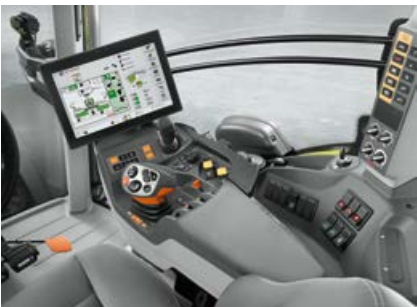
If the tractor is equipped with an ISOBUS-compatible terminal, preselected functions for the CONTOUR can be operated from there
