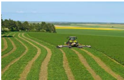
Optimum results even in curves, thanks to maximum overlap (up to 60 cm)
