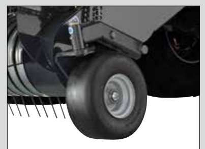
Semi-pneumatic pivoting pick-up guide wheels
