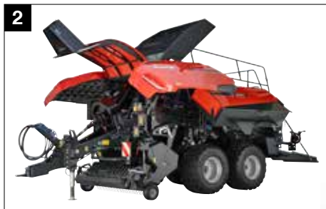
2 Pivoting twine boxes for easy maintenance
