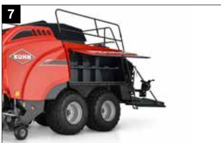
Easy accessible twine boxes with 2x16 capacity
