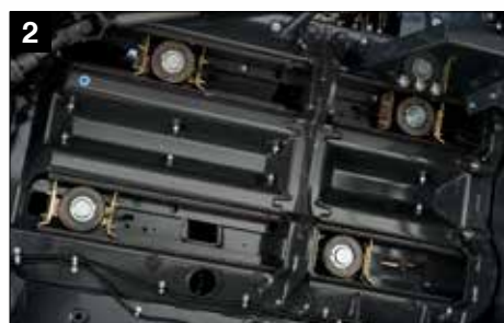
2 Heavy-duty, greased plunger rolls
