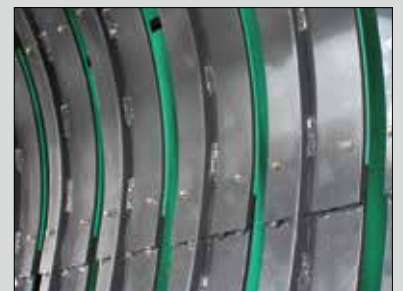
Easy flow plates for pre-chamber
