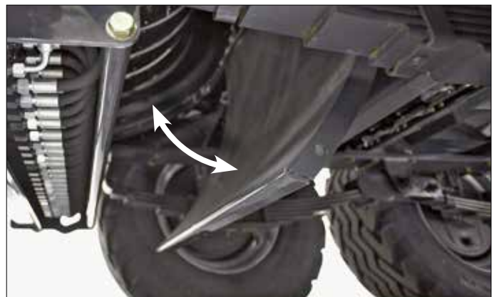
Pre-chamber inspection door
