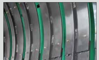
Easy flow plates for pre chamber
