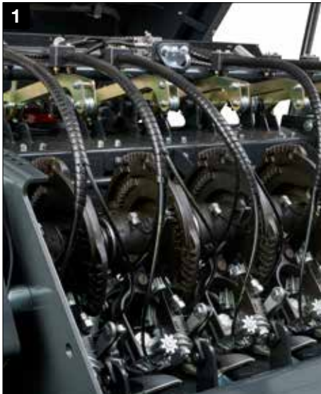
Double knotting system with standard electronic monitoring
