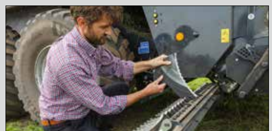
One-sided sliding knife cassette system
