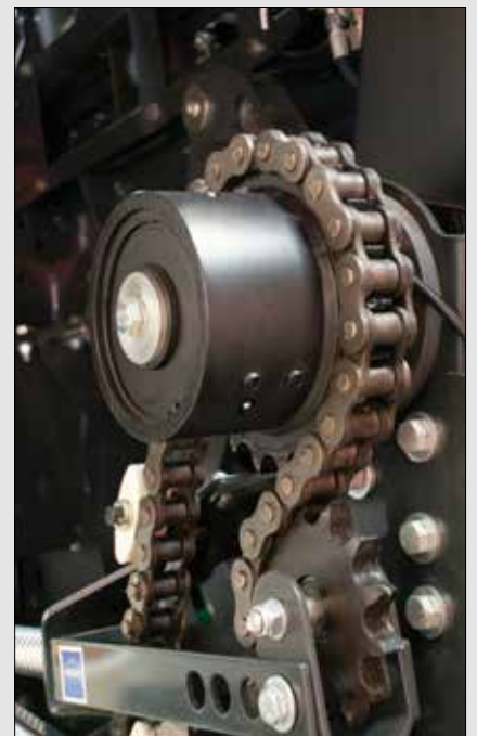
INTEGRAL ROTOR protection clutch
