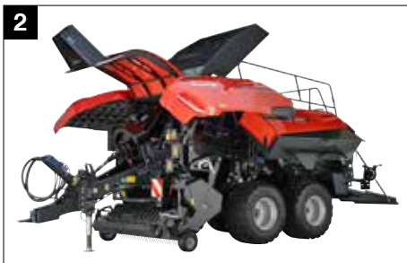
Pivoting twine boxes for easy maintenance
