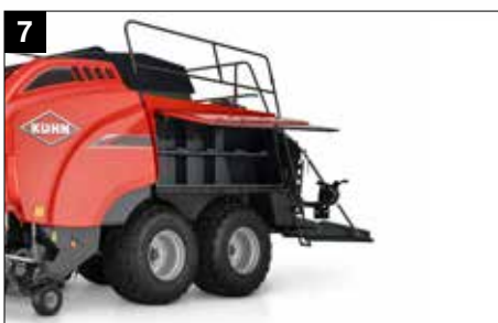
Easy accessible twine boxes with 2x16 capacity
