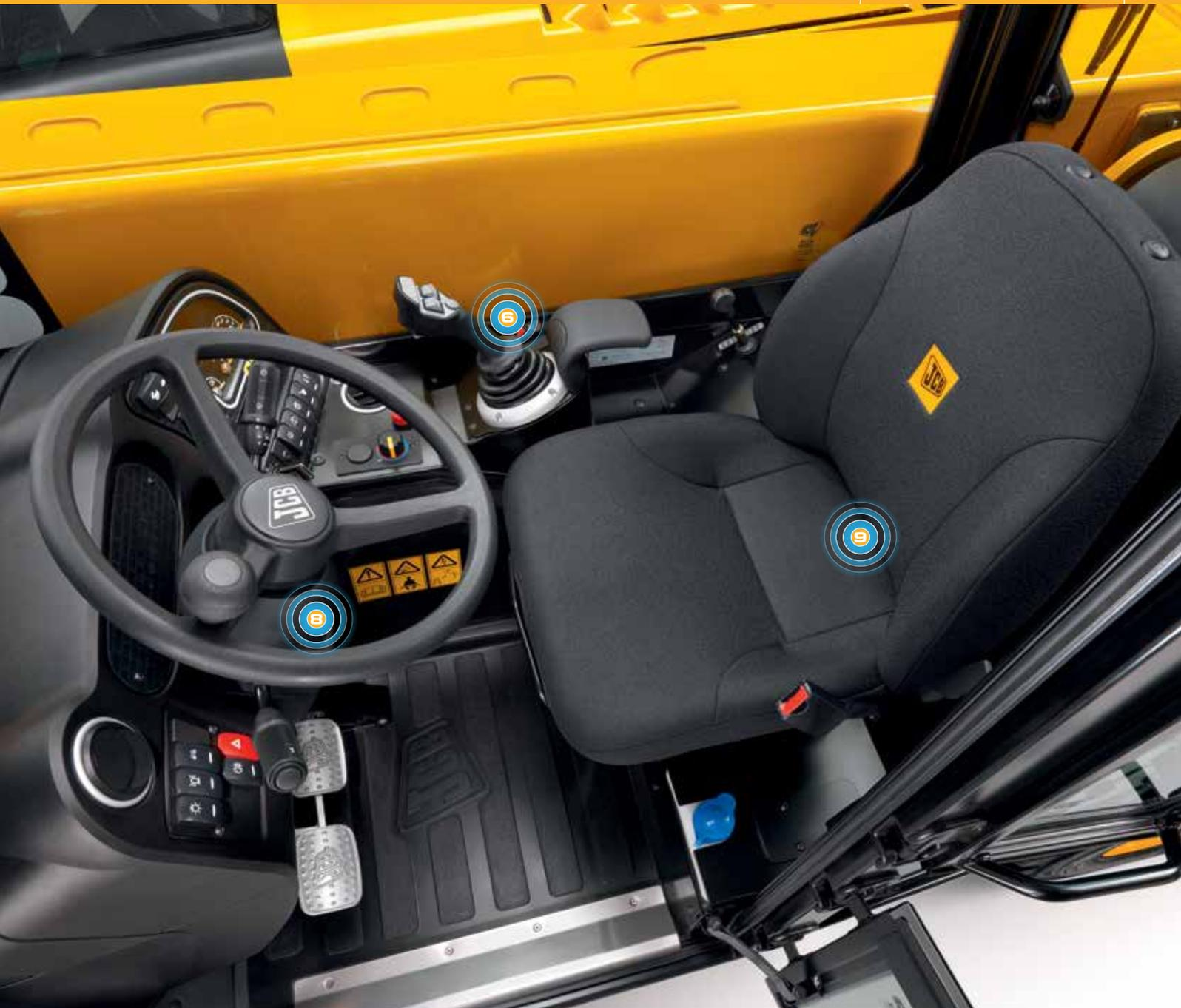
**E** Controlling a JCB 525-60 Hi Viz is comfortable, precise and smooth: there are single lever electro servo controls with proportional auxiliaries.
