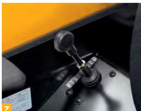
**7** This Loadall has three selectable manual 4-wheel steering modes. Two-wheel steer is perfect for roading; four-wheel steer provides great manoeuvrability in tight spaces; and crab steer is designed to edge your Loadall either close to or away from walls and buildings.
