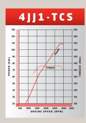
4JJ1-TCS produces 110kW power and 375Nm torque and is standard on NLR, NLS and NNR models.
