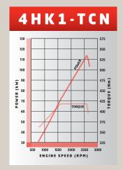
4HK1-TCN produces 114kW power and 419Nm torque and is standard on NPR 45/55 and NPS models.
