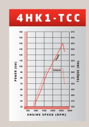
4HK1-TCC produces 140kW power and 513Nm torque on selected NPR models and is standard on NOR models.
