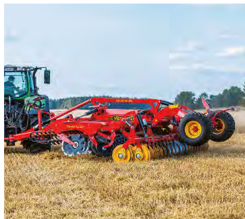
On headlands, the machine can be turned on either the packer or the wheels.
