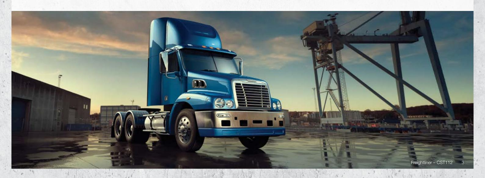
An extremely 'slippery' cabin profile allows the CST112 and its load to better cut through the air, with key design features including its 16 degree sloped bonnet, concealed air intakes and exhausts, a wind-cheating mirror design.
