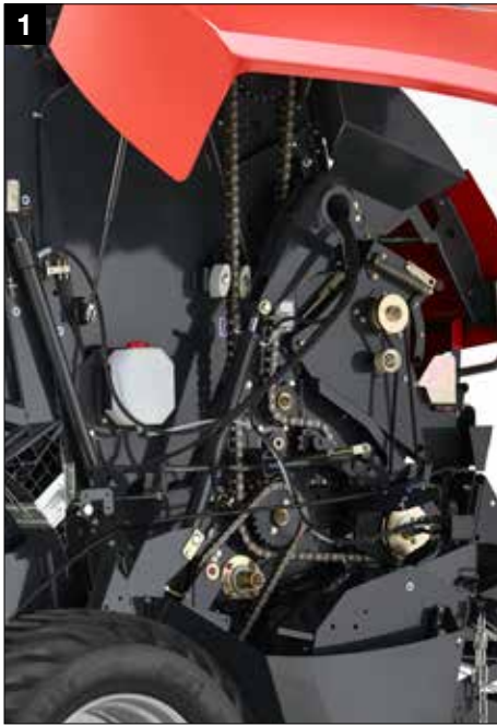
Robust driveline with high-quality IWIS chains
