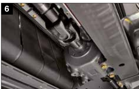
Heavy-duty cross joints in the drive axles
