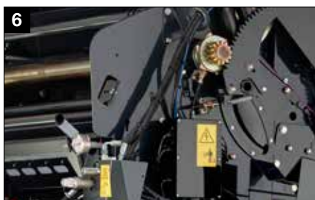
Proportional valve for in-cab density control
