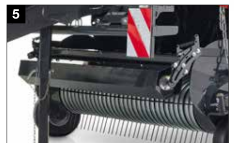
5 Heavy crop roller with wind guard (Ø 217 mm)
