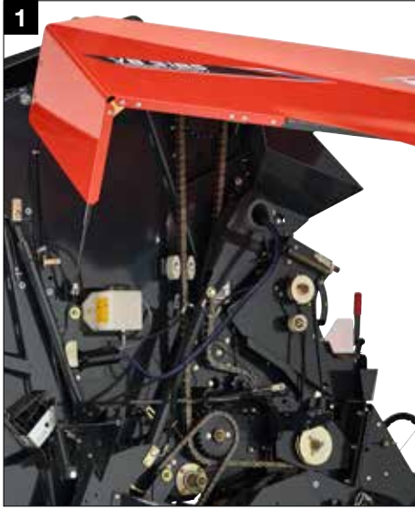
Robust driveline with high-quality IWIS chains
