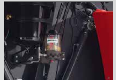
Automatic greasing system
