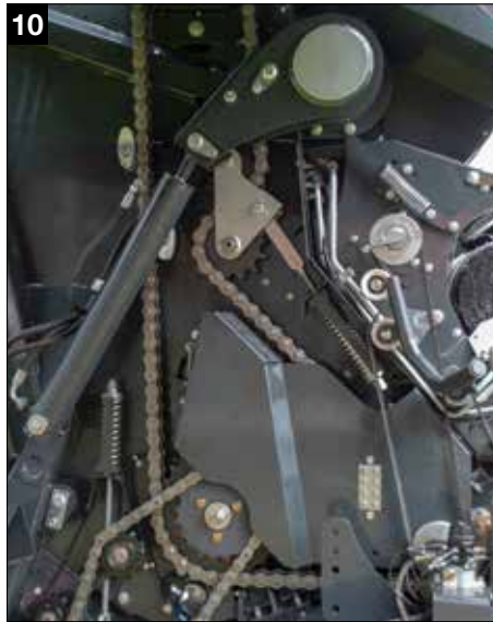
10 Robust driveline with wear-resistant and oversized chains
