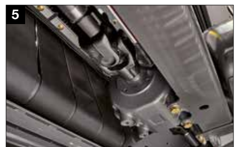
Heavy-duty cross joints in the drive axles
