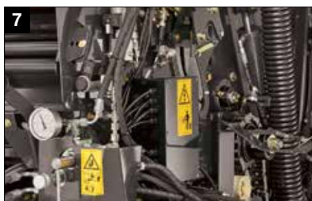
Proportional valve for in-cab density control
