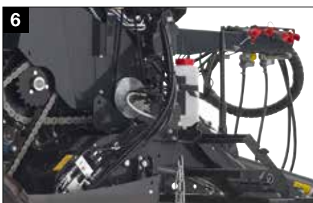
6 BEKA-MAX continuous chain oiling system
