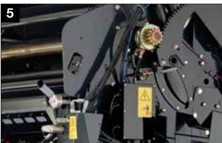
Proportional valve for in-cab density control
