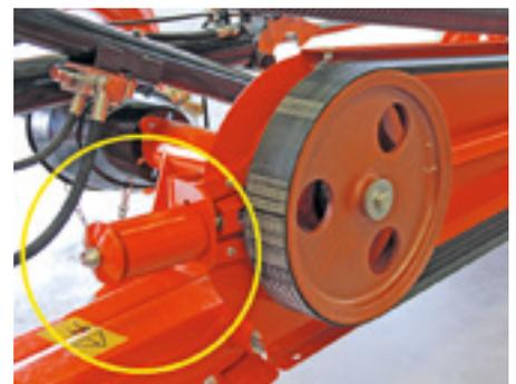
The belt is assembled with a pre-tensioning device avoiding daily intervention. The distribution of the greasing points has also been optimized to limit maintenance time. Greasing operations are limited to the transmission and one other point. All other machine pivot points are mounted on ORKOT bushings with hard chromed axes, which do not require lubrication. This precious time saved can then be allocated to other work.
