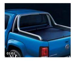
**O1** Roll cover. The lockable load compartment cover protects the cargo from prying eyes.
