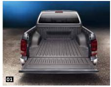
Cargo area coating. The UV-resistant special coating in anthracite provides excellent protection against mechanical and chemical wear. | UL |
