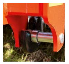
**1.** A wide range of drawbar linkage categories is available (categories 3, 4N, 4, K700 and QuickCoupler 3 and 4N) to adapt to medium and high power tractors (135 to 360 hp). For more modularity, the spacers can be changed in order to change category !
