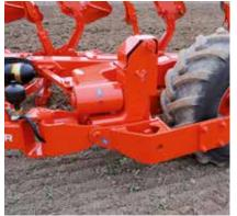
**5.** A large sized wheel (500 x 1000 mm or 500 x 1200 mm) supported on both sides ensures stability in U-turns and provides a longer hub life !!
