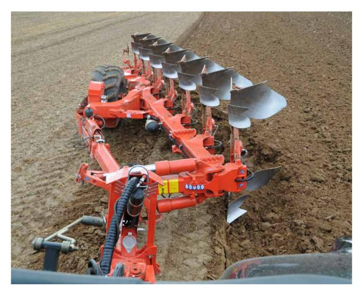
For additional serenity, this variable width system is maintenance-free. All pivot points are stopped from rotating and fitted with bushes.
