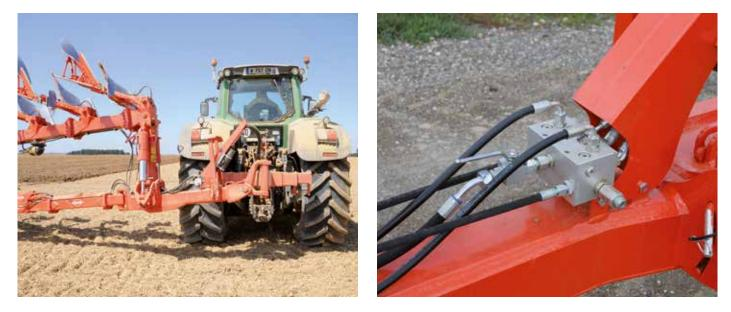
For your comfort : fewer spool valves to operate in U-turns as the entire range is equipped with hydraulic sequencing as standard.
