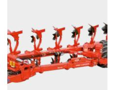
**4.** For added serenity, the structure is made robust by a large dimensioned machine-welded frame =  $180 \times 180$  mm.
