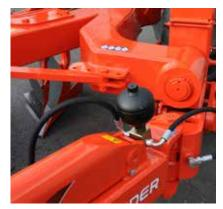
**6.** For more stability in transport as well as frame protection during road and path travel, the lifting cylinder is equipped with hydro-pneumatic suspension.
