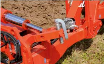
**1. Levelling :** by independent left / right crank screws for extra precision.
