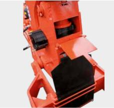
**2. Depth :** by spacers on the lift cylinder. All stress is axial = no constraint on the pivot pins. The number of spacers gives the point of reference.
