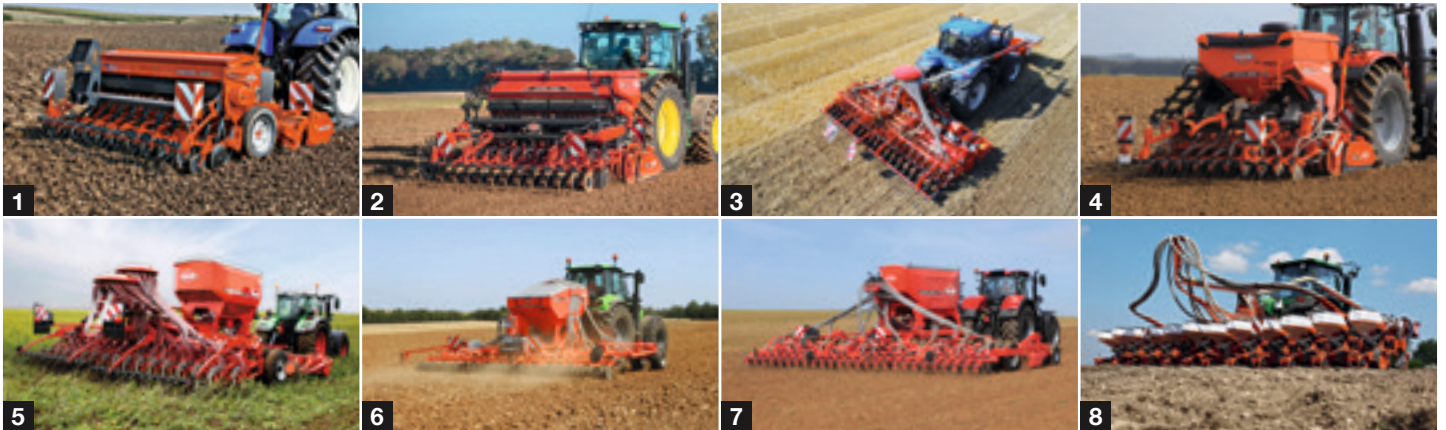
1. mounted mechanical 2. integrated mechanical 3. with front hopper 4. integrated pneumatic 5. trailed pneumatic 6. mounted for min-till 7. trailed for min-till 8. precision seed drills
