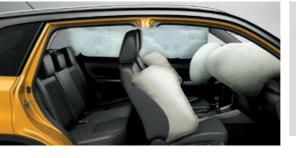
The Vitara's body design centres on Suzuki's TECT Driving performance is complemented by protective safety features, including standard SRS airbags for the absorbs and disperses the energy in the event of driver and front passenger, front SRS side airbags that reduce impact to the chest in side collisions and SRS curtain airbags that reduce impact to the head.
