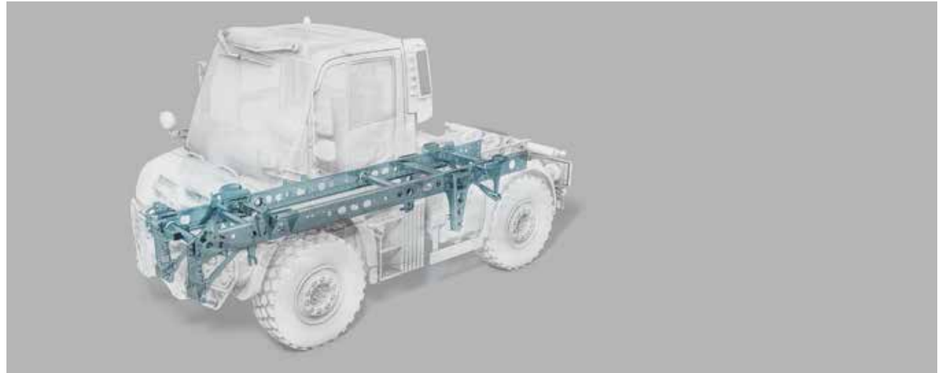
Four attachment and mounting areas: the Unimog implement carrier is one of the most productive work vehicles there is. Many different implements can be combined thanks to the standardised interfaces. These include the front mounting plate, attachment points on the frame, mounting brackets on the sides and at the rear as well as ball-point positions on the platform sub-frame.
