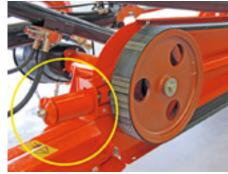
The belt is assembled with a pre-tensioning device avoiding daily intervention.
