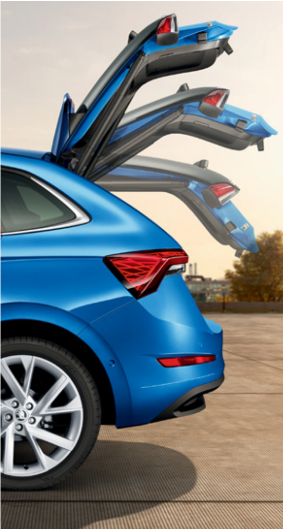
AUTOMATIC TAILGATE It opens and closes at the mere touch of a button on the remote control or in the driver's door, especially handy in unfavourable weather. You can also adjust the upper door position to suit your needs. A button for closing the 5th door is also located on the door itself.
