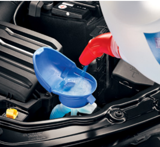
LIQUID RESERVOIR You will never spill a single drop when refilling the washer fluid. The liquid reservoir is not only easily accessible, but also has an integrated funnel.
