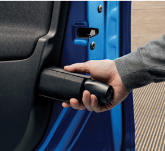
UMBRELLA STORAGE COMPARTMENT An ingenious compartment with original ŠKODA umbrella is fitted inside the driver's door. It is designed to let water drain away from the car, keeping the interior dry.
