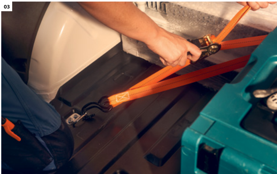
03 Lashing eyes. Keep their promise. The six folding lashing eyes secure heavy loads rock-solid on the vehicle floor of the new Caddy Cargo. | C |
