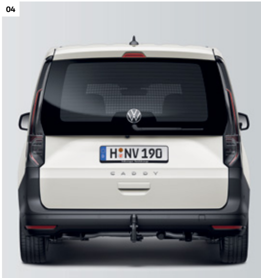
04 Tailgate with window. Opens particularly smoothly and can also be used as a shelter in the rain thanks to its large opening height. The wide window cutout extends the field of visibility. | C | CR |
