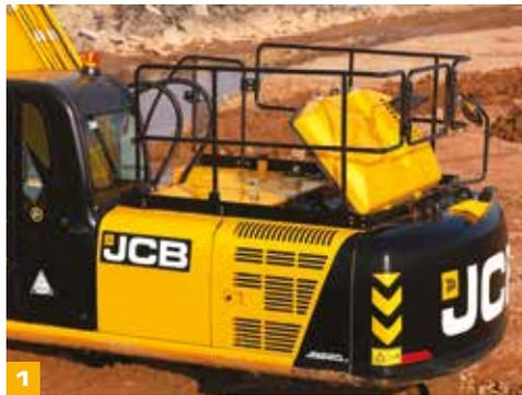
1 The JS220 bonnet opens front-to-rear for easy and safe engine service access.
