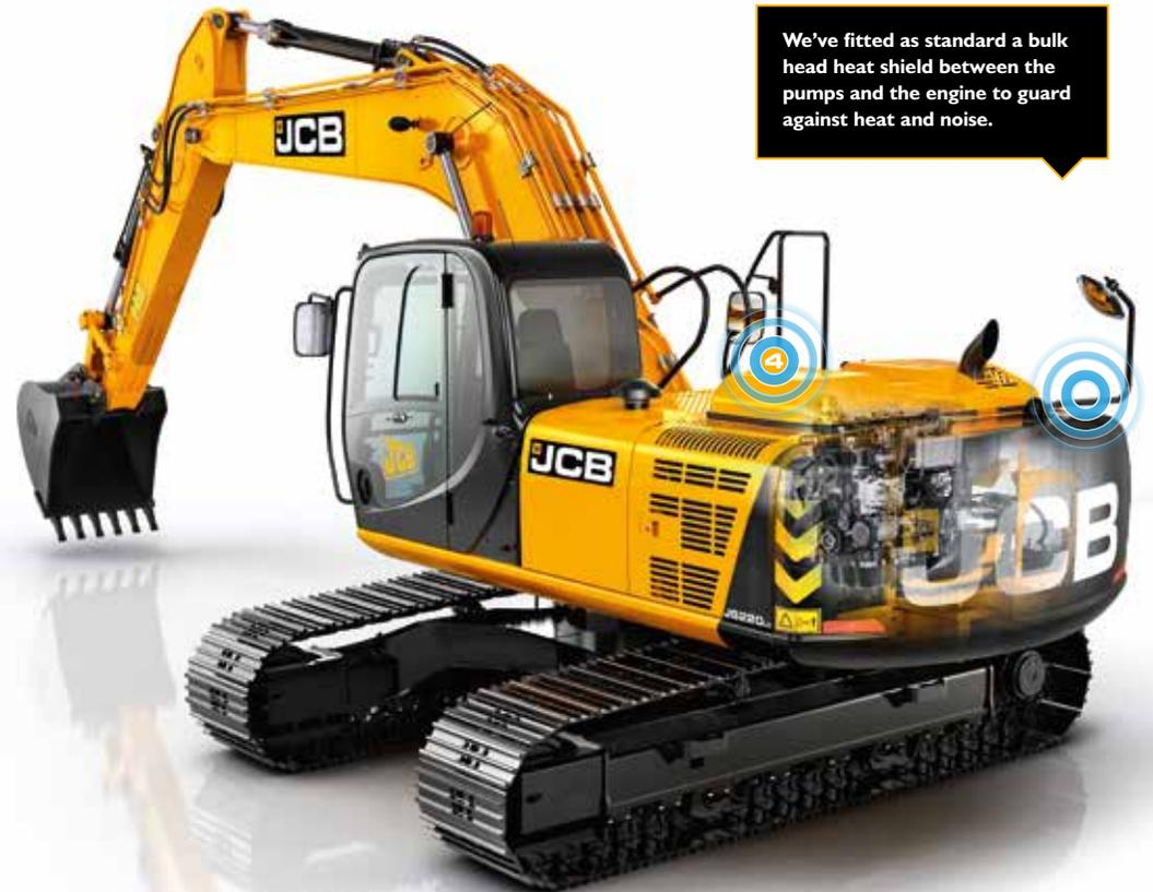
We've fitted as standard a bulk head heat shield between the pumps and the engine to guard against heat and noise.
