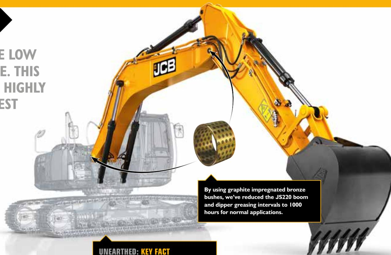
By using graphite impregnated bronze bushes, we've reduced the JS220 boom and dipper greasing intervals to 1000 hours for normal applications.
