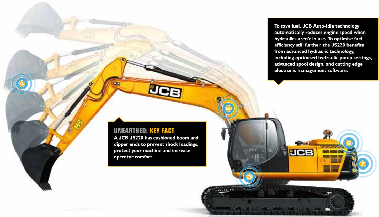
To save fuel, JCB Auto-Idle technology automatically reduces engine speed when hydraulics aren't in use. To optimise fuel efficiency still further, the JS220 benefits from advanced hydraulic technology, including optimised hydraulic pump settings, advanced spool design, and cutting edge electronic management software.
