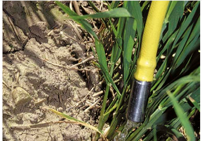
✔ Drag hose kit with stainless steel weights
