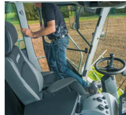
The seat contact switch automatically switches off the front attachment and main drive
