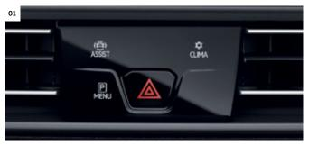
01 Direct access button module. The module is arranged centrally around the hazard warning lights button and uses shortcuts for easy access to major functions such as driver assistance systems, air conditioning functions and parking assistance systems. |C|L
