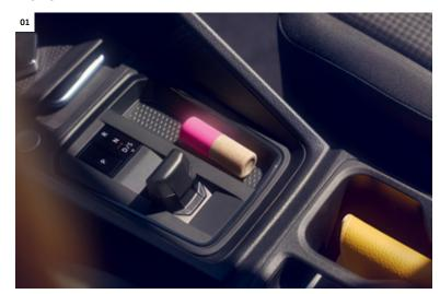
O1 Dual-clutch gearbox (DSG). The Caddy is fitted with an adaptive 7-speed dual-clutch gearbox. This enables fully automatic, smooth gear changes without interruption of tractive power, and it also adapts to the driver's driving style. You can also shift up and down using rocker switches on the steering wheel. |C|L|
