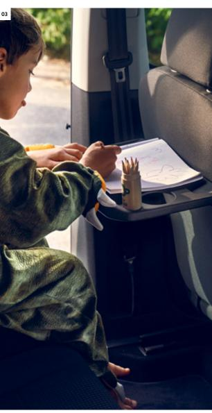
**03** Folding tables in the passenger compartment. Folding tables are built into the front seat backrests. They provide a practical surface and an integrated drink holder for passengers in the second row of seats. | C | L |
