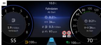
O3 Digital Cockpit Pro. A full digital dashboard experience allowing personalisation of key functions and information. Customised views show data on audio, phone, consumptions and if optioned, navigation. Display content can be adjusted using the steering wheel controls.
