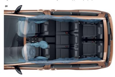
**09 Front, side, curtain and centre airbags.** The Caddy is equipped with one front airbag for the driver and one for the passenger. Centre airbags prevent a collision between the driver and front passenger. And curtain airbags offer all passengers sitting on the outer seats protection in the event of a side-on collision. | C | L |
