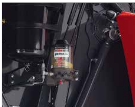
10. Automatic greasing system
