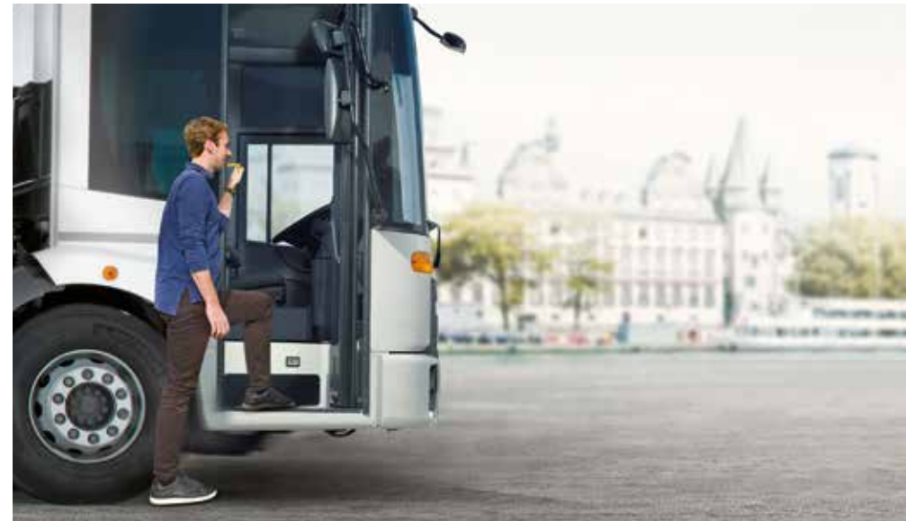
Two steps for improved ergonomics: the low-entry design of the Eonic makes getting in easier and getting out safer.
