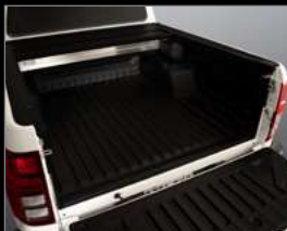
Under Rail Tub Liner
