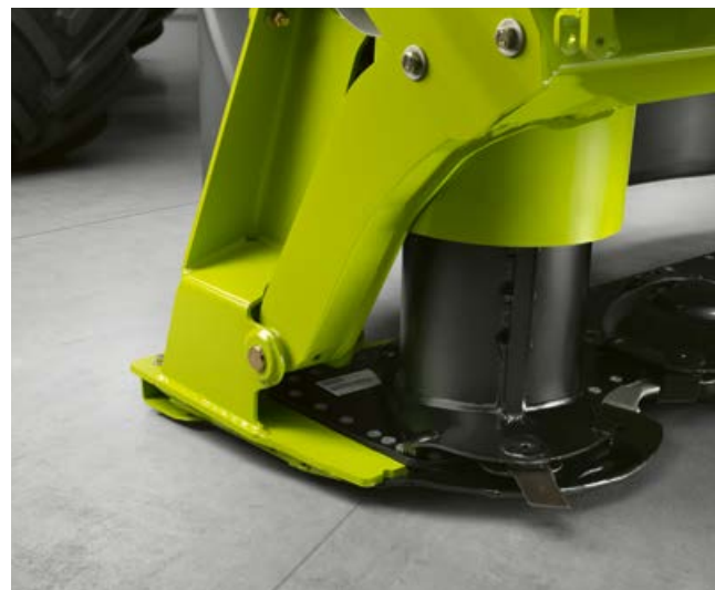
Sophisticated linkage geometry for outstanding ground-contour following.
