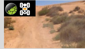
4LLC (4WD Low Range with locked centre differential) For steep hills, sand, deep snow, etc.
