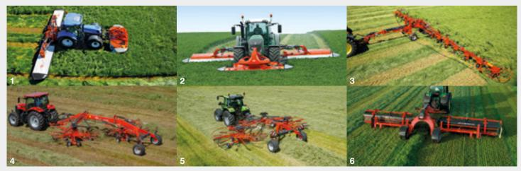
1. Triple disc mowers - 2. Triple disc mower conditioners - 3. Trailed gyro tedders with 13 and 17 m working width - 4. Semi-mounted twinrotor gyro windrowers with side delivery - 5. Semi-mounted twin-rotor gyro windrowers with central delivery - 6. Conveyor belt windrowers
