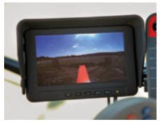
**Obtain an overview** A camera mounted on the rear of the rake provides an overview from the cab. The machine is safe and easy to use at work, on the road and when turning.
