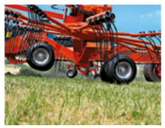
A very useful "jet" effect Just like an aeroplane, the rear of the rotor lands before the front of the rotor, The tines therefore do not come into contact with the soil, thus preserving the plant cover and avoiding tine wear and breakage.
