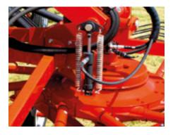
**Stable at work and on the road** With the STABILIFT system, available only on the GA 13231 and GA 15231 models, a hydraulic cylinder automatically locks the rotor articulation once it is raised. The machine becomes more stable.
