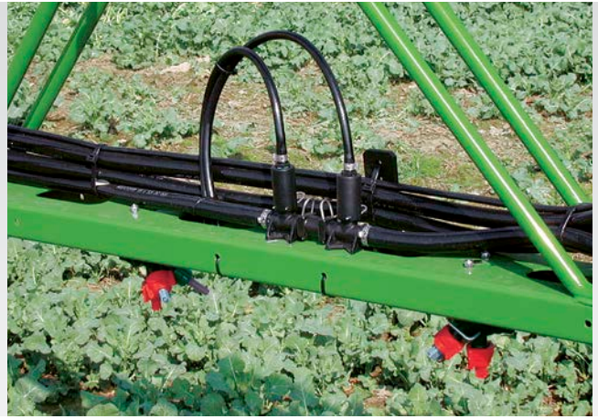
DUS pressure recirculation system
