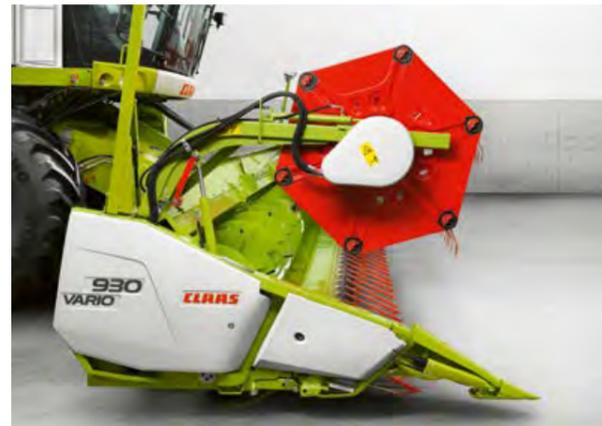
Cutterbar table retracted – grain (- 100 mm)
