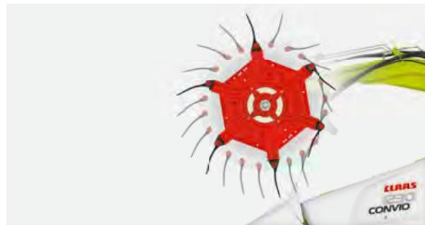
Cam-track-controlled reel with flip-over concept
