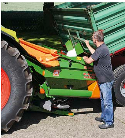
Filling with tipping trailer
