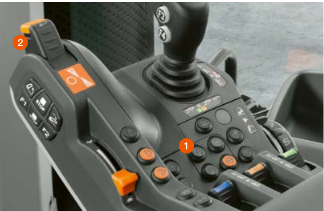
CIS+ operation 1 Change range 2 Activate cruise control
