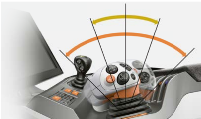
Shifting operation, powershift speeds + / - Shifting operation, range + / -
