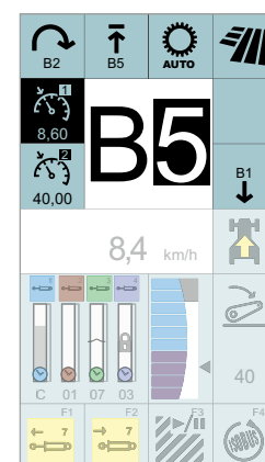
Intelligent gear selection on the A-pillar display in the CIS version.
