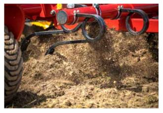
The vibrating Swift tines deliver an intensive mixing down to 7.75" (20 cm) working depth.
