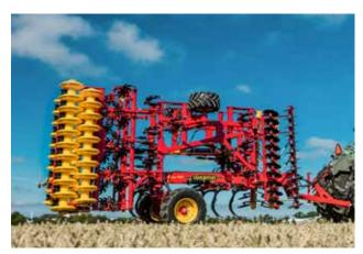
TopDown 300-700 folds to 10' (3 m) transport width, while the wider TopDown 900 folds to 16.5' (5 m).
