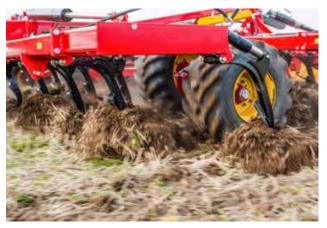
The powerful Opus tines are equipped with a stone release with up to 1545 lbs (700 kg) release force. This ensures depth is maintained down to 15.75" (40 cm) working depth.
