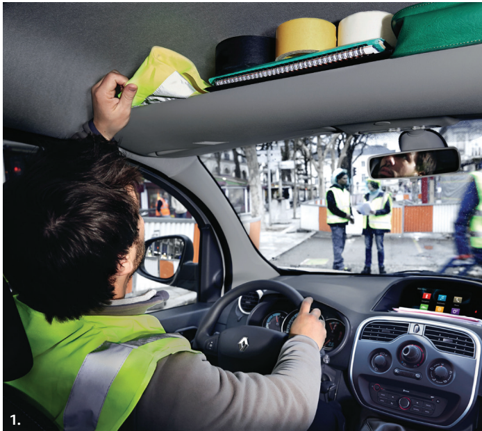
1. Roof storage rack. With storage space above the windscreen, the roof panel rack is wide and deep enough to store a range of items.
