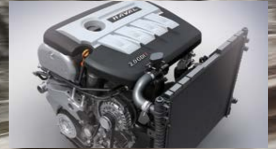
Powerful 145kW turbo-charged 2.0-litre direct injection engine
