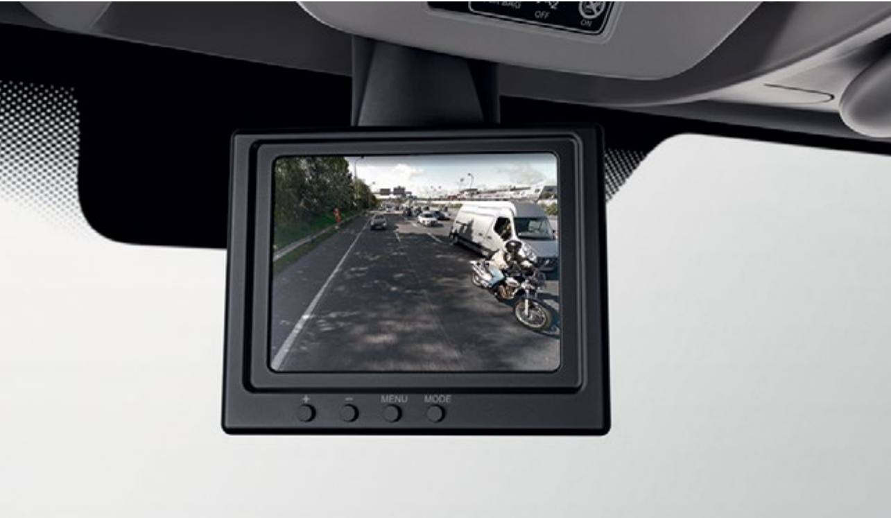
smart rear-view mirror* Using a rear-mounted camera, it provides excellent medium and long-distance vision of the surroundings via an in-cab digital display.
