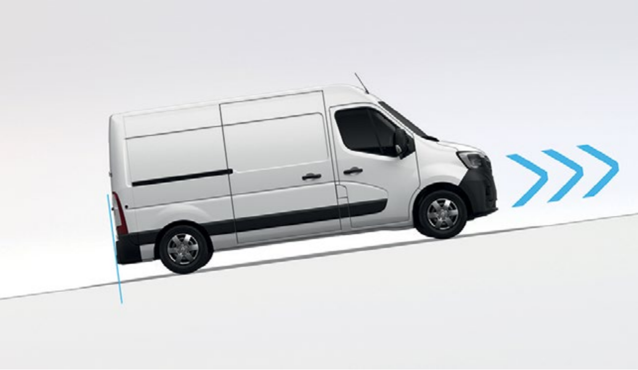
hill start assist Combined with ESC, hill start assist maintains brake pressure automatically for 2 seconds to give you time to lift your foot from the brake pedal and press the accelerator. The system activates when the slope exceeds 3%.
