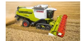
The new hydropneumatic suspension provided a high level of driving comfort in the field and on the road. This crawler track system is still fitted today.
