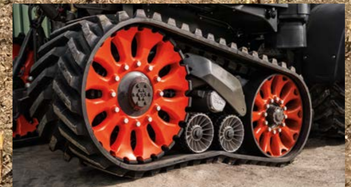
The independent suspension of the drive wheel, land wheel and support rollers allows the crawler track unit to adapt optimally to the ground surface.
