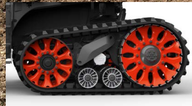
The large drive wheel allows high torque transmission.
