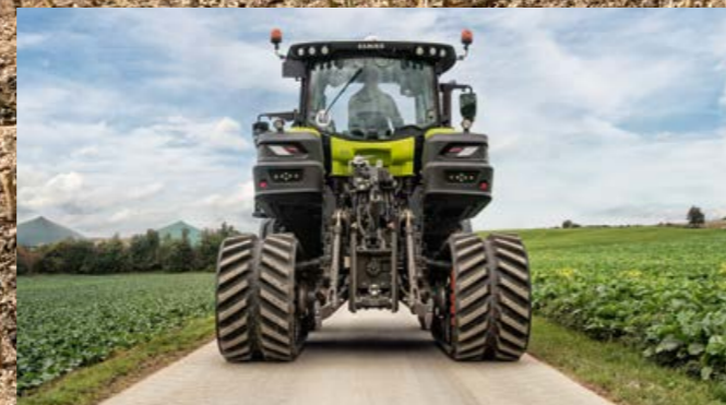
Despite its large contact area, the AXION 900 TERRA TRAC is narrower than the version with wide or twin tyres.
