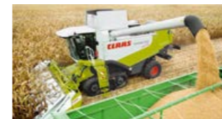
The track units were now suspended on the axle by rubber blocks. This led to significantly reduced impact loads on the machine and a high level of driving comfort.
