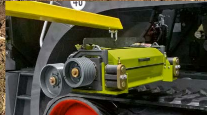
Good accessibility: possible to remove corncripper from the side above the crawler track
