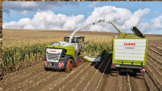
Low rut formation improves accessibility for all the other vehicles in the crop handling chain
