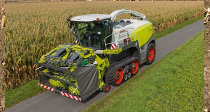
With the 635 mm wide track, the JAGUAR has an external width of 2.99 m
