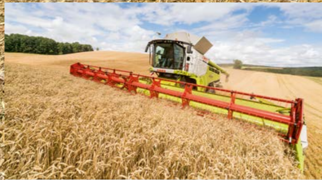
With wide front attachments in particular, the TERRA TRAC crawler tracks make a major contribution to smooth and steady cutterbar guidance.
