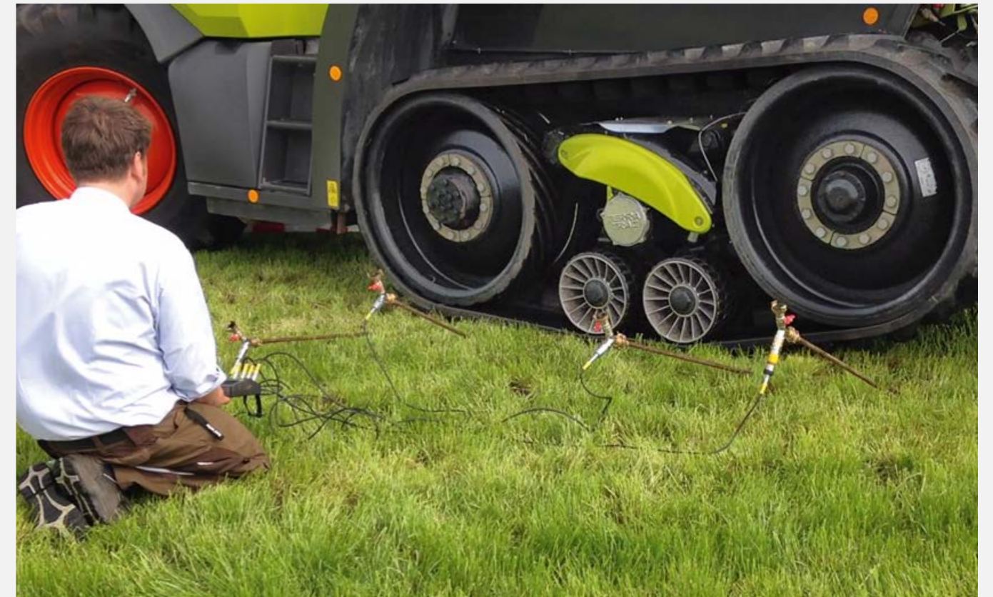
Measurement of soil pressure during cornering with headland protection
