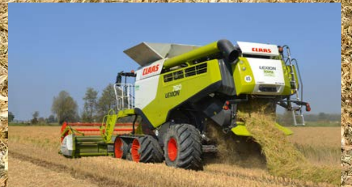
For the four different LEXION models a total of four different TERRA TRAC tracks are available in three widths: 635 mm, 735 mm as well as 890 mm for grain and 890 mm for rice.
