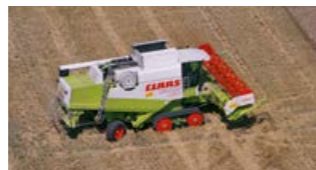
The first TERRA TRAC crawler track series on a LEXION 450 was still attached rigidly to the axle. The land wheels were made of steel with bolted-on rubber elements to withstand the high frictional loads.
