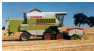
CLAAS started TERRA TRAC trials with a MEGA combine harvester. The land wheels had pneumatic tyres.
