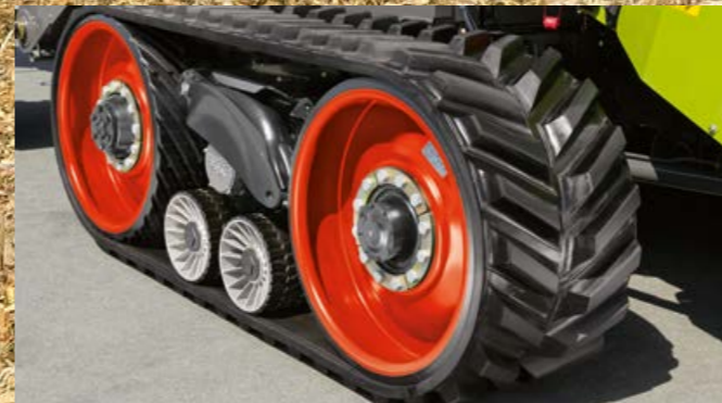
New track: the newly developed track with a modified rib layout is able to withstand the heavy loads encountered during on-road operation for longer.
