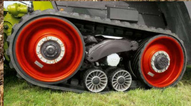
Headland protection: track contact area is shortened automatically by lifting the land wheels when cornering
