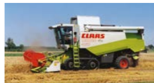
For the US market, the combine harvesters were equipped with vulcanised land wheels as well as improved tracks which brought a further increase in their durability.
