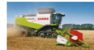
The TERRA TRAC crawler track units now had a significantly reinforced structure thanks to a one-piece cast frame in order to meet the demands of the increased weight of the machines.
