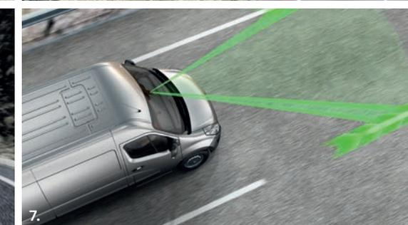
1. Driver and passenger airbags 2. Rear parking sensors and camera 3. ABS with EBD 4. Adaptive ESC and Traction Control 5. Cruise control and speed limiter 6. Cornering lights\* 7. Lane Departure Warning\*
