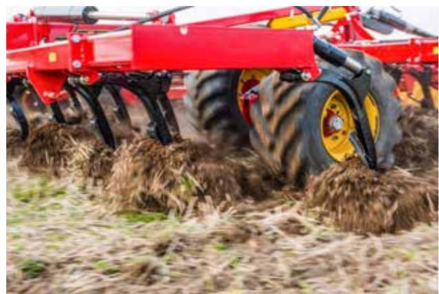
*The powerful Opus tines are equipped with a stone release with up to 1545 lbs (700 kg) release force. This ensures depth is maintained down to 15.75" (40 cm) working depth.*
