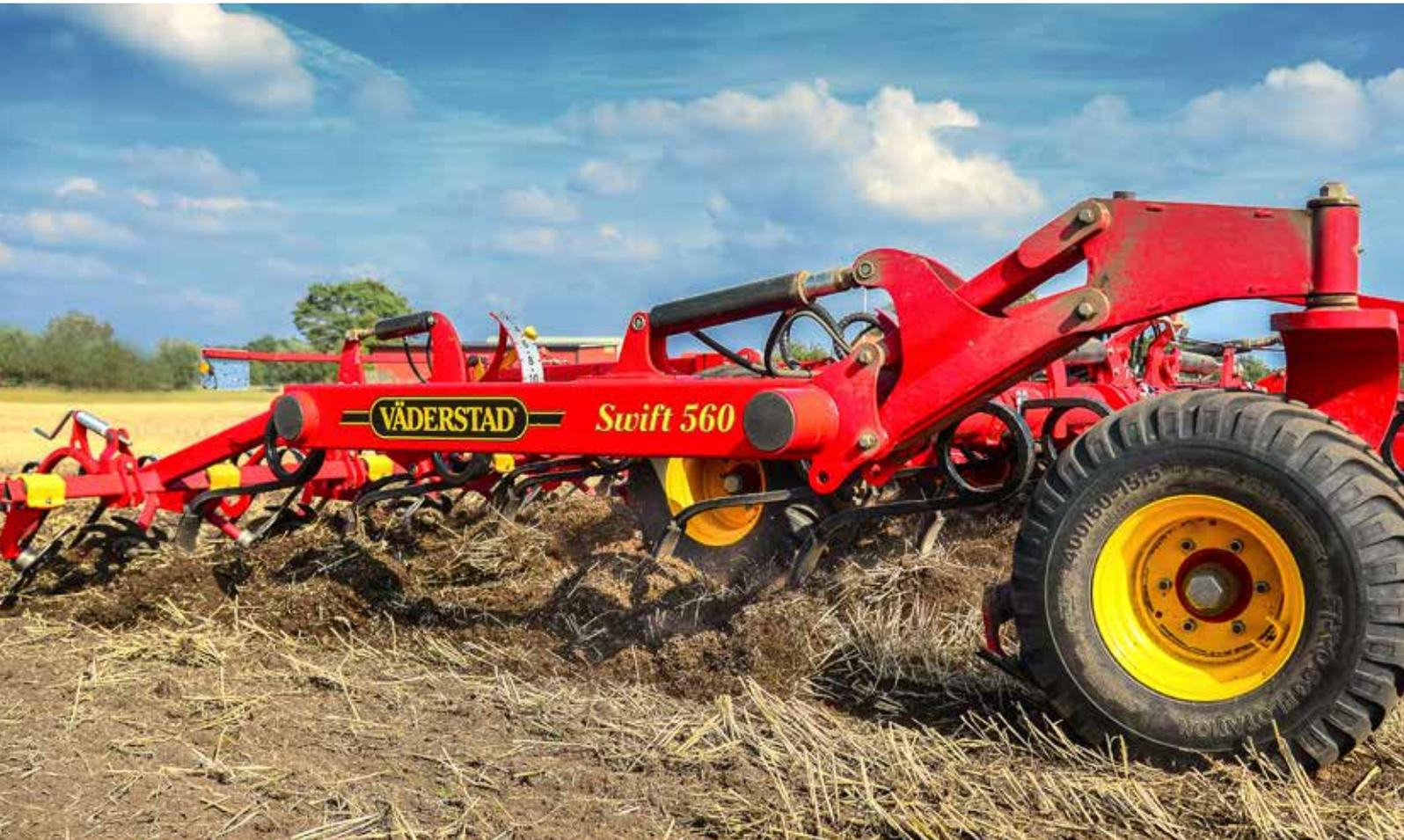
The models in the product family span from 13-28.5' (4- 8.7 m) working widths.
