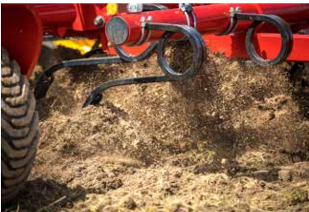
*The vibrating Swift tines deliver an intensive mixing down to 7.75" (20 cm) working depth.*
