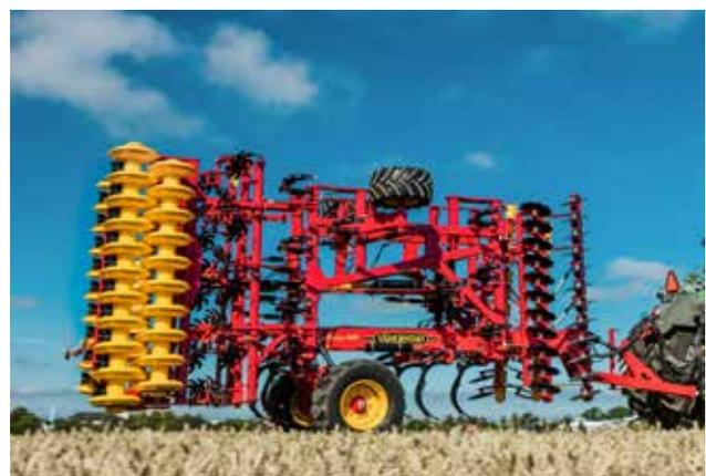
*TopDown 300-700 folds to 10' (3 m) transport width, while the wider TopDown 900 folds to 16.5' (5 m).*
