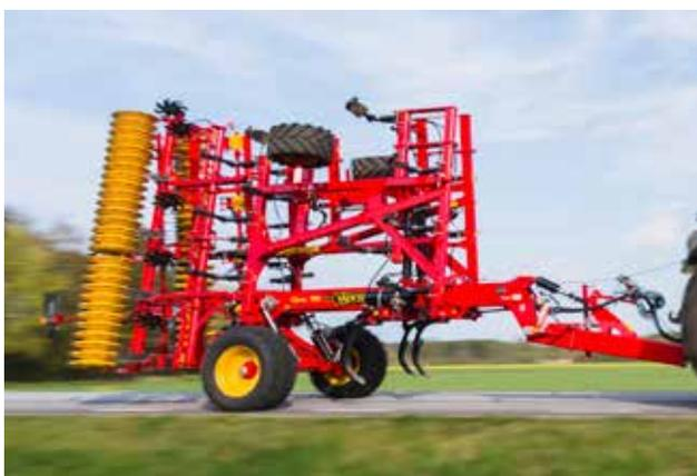
*The carrying wheels positioned in the middle of the machine, makes Opus both easy to transport and gives it a small turning radius on headlands.*
