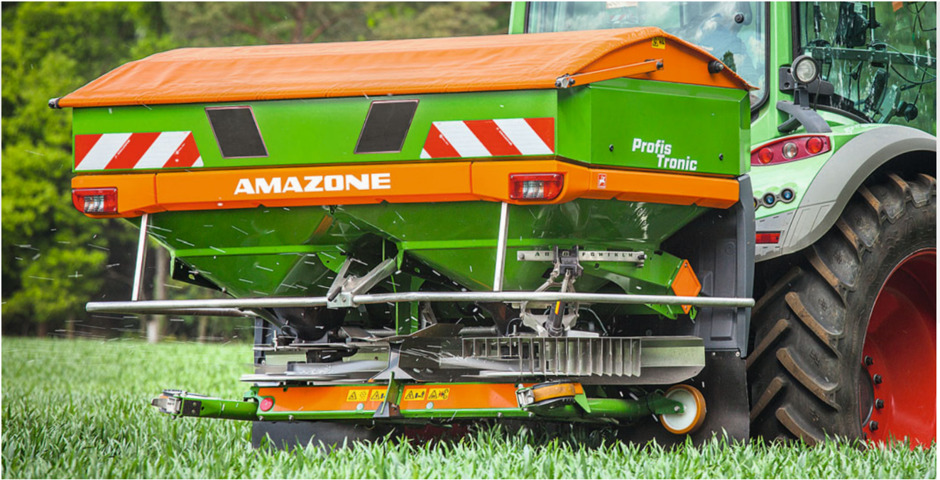
Border spreading with activated Limiter V +
