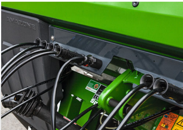
Accessible holder for the hydraulic hoses
