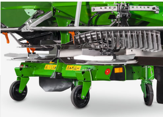
Special frame with rolling and parking device
