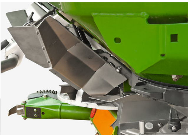
Border spread deflector folded upwards
