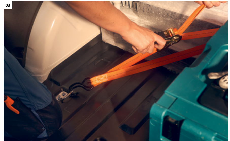
03 Lashing eyes. Keep their promise. The six folding lashing eyes secure heavy loads rock-solid on the vehicle floor of the new Caddy Cargo. | C |
