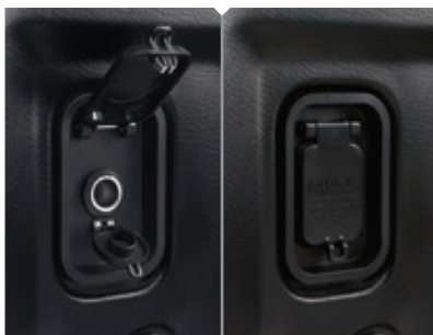
Deck power outlet
