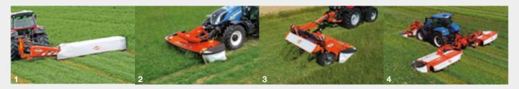
1. Rear-mounted mowers - 2. Front-mounted disc mowers - 3. Trailed disc mowers - 4. Triple gang disc mowers
