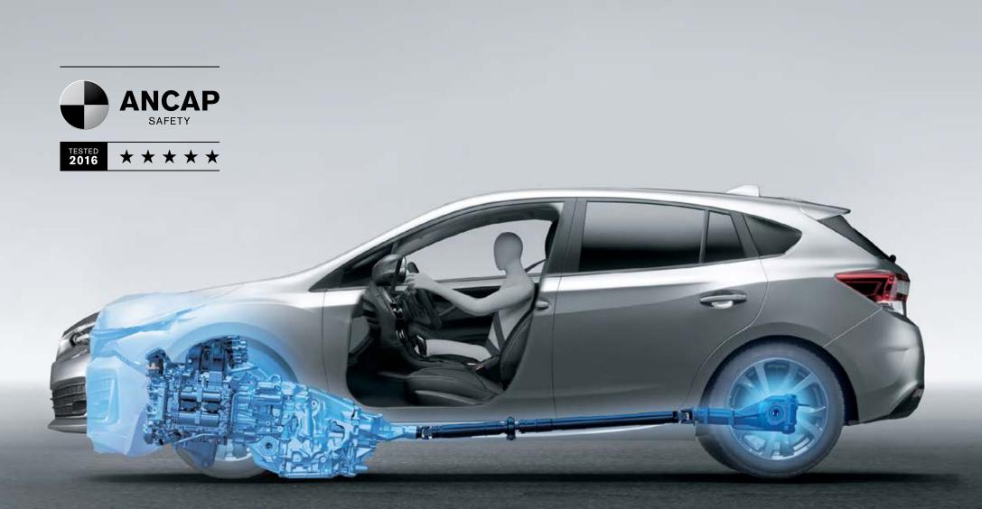
Designated crumple zones direct impact energy away from the ring-shaped passenger safety cell, while the Boxer engine is designed to slide below the cabin in a severe frontal collision.
