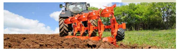
The MASTER 153 ploughs have been designed to meet the same requirements as the 123 series, but are designed for more intensive use and more difficult working conditions with more powerful tractors ranging from 95 to 270 hp.
