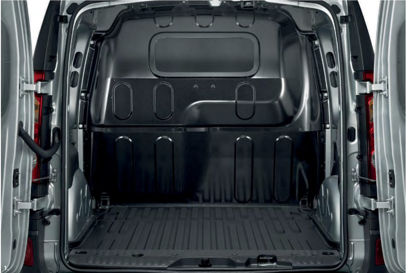
1. Steel bulkhead. Fully isolates the loading space from the driver's position.
