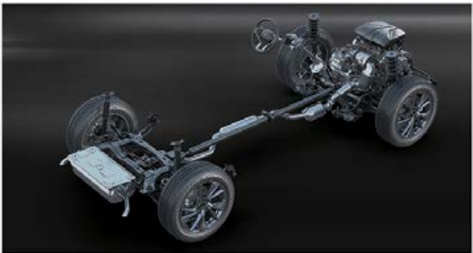
Front Macpherson Rear Multi-link Independent Suspension + AWD
