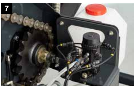
BEKA-MAX continuous chain oiling system
