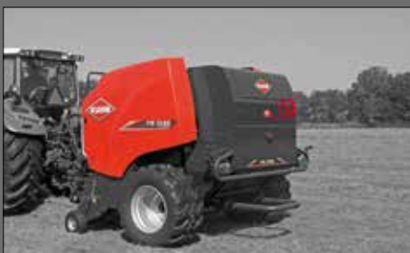
Net binding is being applied, visual and acoustic signals on the baler are activated
