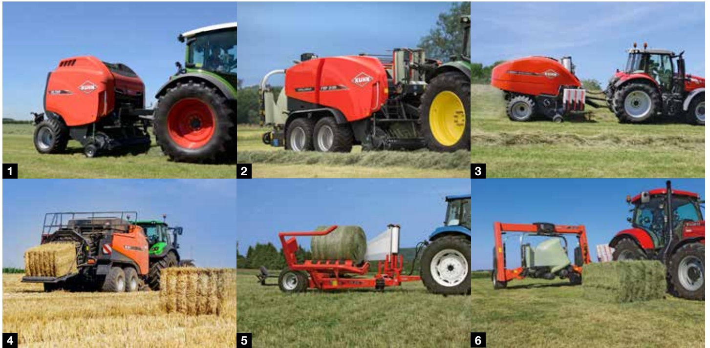
1. Variable Balers - 2. BalePacks - 3. i-BIO+ - 4. Large Square Balers - 5. + 6. Round and Square Bale Wrappers.
