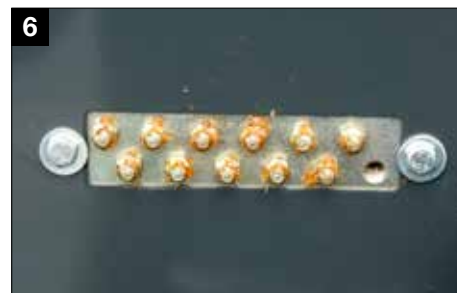
Centralized grease banks for roller bearings
