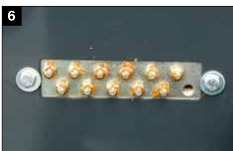
Automatic chain lubrication and centrally located grease banks for roller bearings
