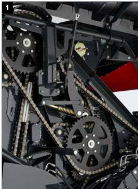
Robust driveline with high quality IWIS chains
