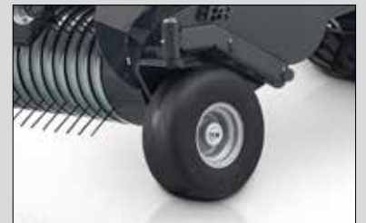
Pivoting semi-pneumatic pick-up guide wheels
