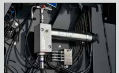
Automatic greasing system for roller bearings
