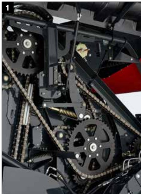
Robust driveline with high quality IWIS chains
