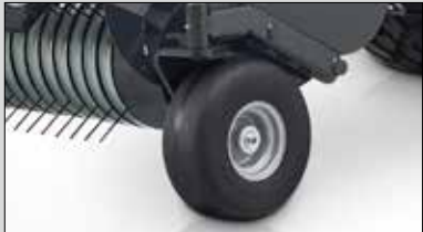
Pivoting semi-pneumatic pick-up guide wheels
