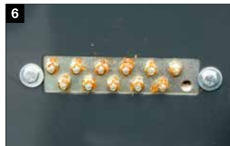
Centralized grease banks for roller bearings
